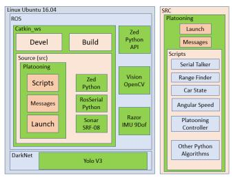
Fig. 3. Software Architecture
