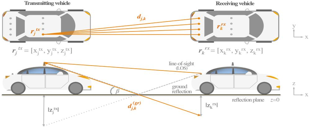
Fig. 1: V2V communication link showing: (bottom) both the LOS and ground reflected path components that the signals from the transceiver mounted on the transmitting vehicle (left) follow when sent to the receiving vehicle (right), according to the two-ray model; and (top) an aerial view of the V2V channel.
