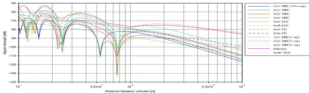
Fig. 5: Received signal strength (dB) vs distance between vehicles for several configurations of multiple antennas at the transmitter and receiver side, considering ground reflected wave propagation, EGC and full diversity.
