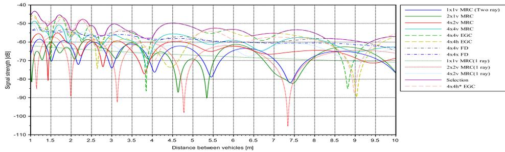
Fig. 3: Received signal strength (dB) vs distance between vehicles for several configurations of multiple antennas at the transmitter and receiver side, considering ground reflected wave propagation, EGC and full diversity.
