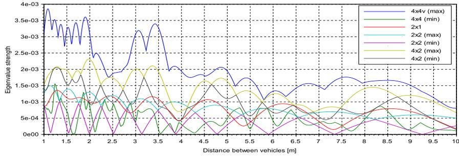
Fig. 2: Maximum and minimum singular values for the channel matrix versus distance between vehicles.
