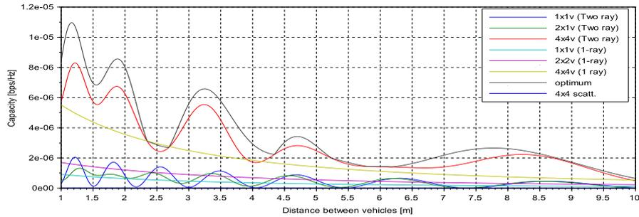
Fig. 4: Capacity (bps/Hz) vs distance between vehicles for several configurations of multiple antennas at the transmitter and receiver side, considering ground reflected wave propagation, EGC and full diversity.
