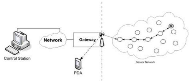
Fig. 1. Topology of a Wireless Sensor Network
