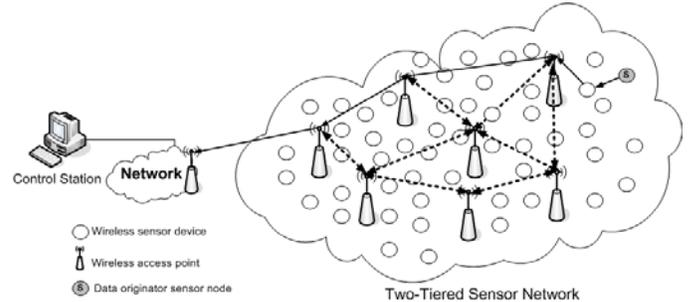
Fig. 2. Two-Tiered Sensor Network Architecture
