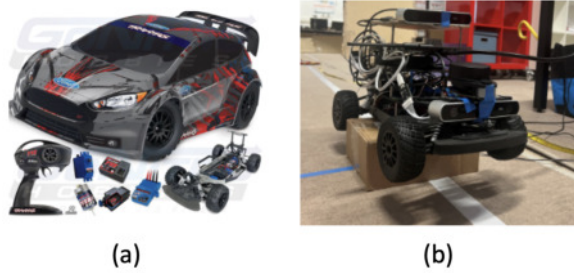
Fig. 3. Traxis Ford Fiesta car model 4(a) and the vehicle model of our test bed with Zed cameras and Lidar installed on it 4(b)
